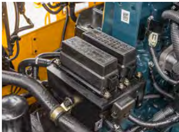
IP67 Class Fuse & Relay box
