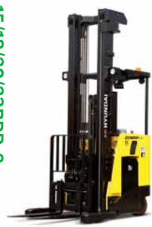
Pantograph Reach Truck 3,000 - 4,500 lbs. capacity
